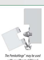
The PemkoHinge<sup>-</sup> may be used with or without additional security hinge bolts.
