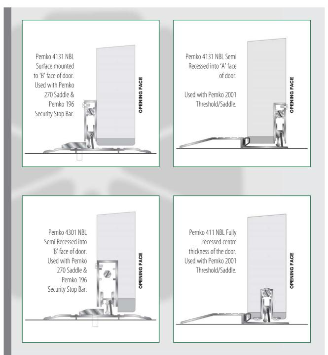
*NOTE: These details illustrate some of the possible applications for the use of Pemko security drop seals. These are intended for use with external opening out doors.*
