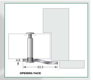
• The Closing Stile Astragal Guard can be used with Steel or Wood doors.
