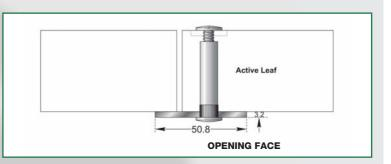
The Pemko 357 Security Astragal is designed to protect against forced entry attack by restricting access to the operating gap at the meeting stiles of pairs of doors.
