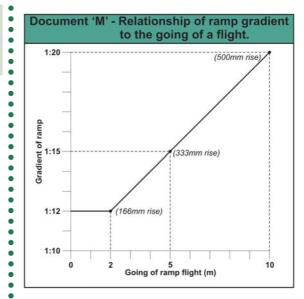
Document 'M' - Limits for Ramp GradientsGoing of a flightMaximum gradientMaximum rise10m1:20500mm5m1:15333mm2m1:12166mm
